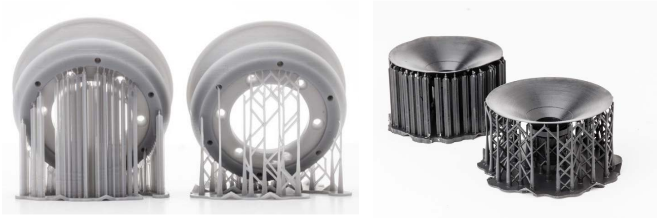
Fig. 7 Different software will have different algorithms for support structures (Baptiste 2018).
