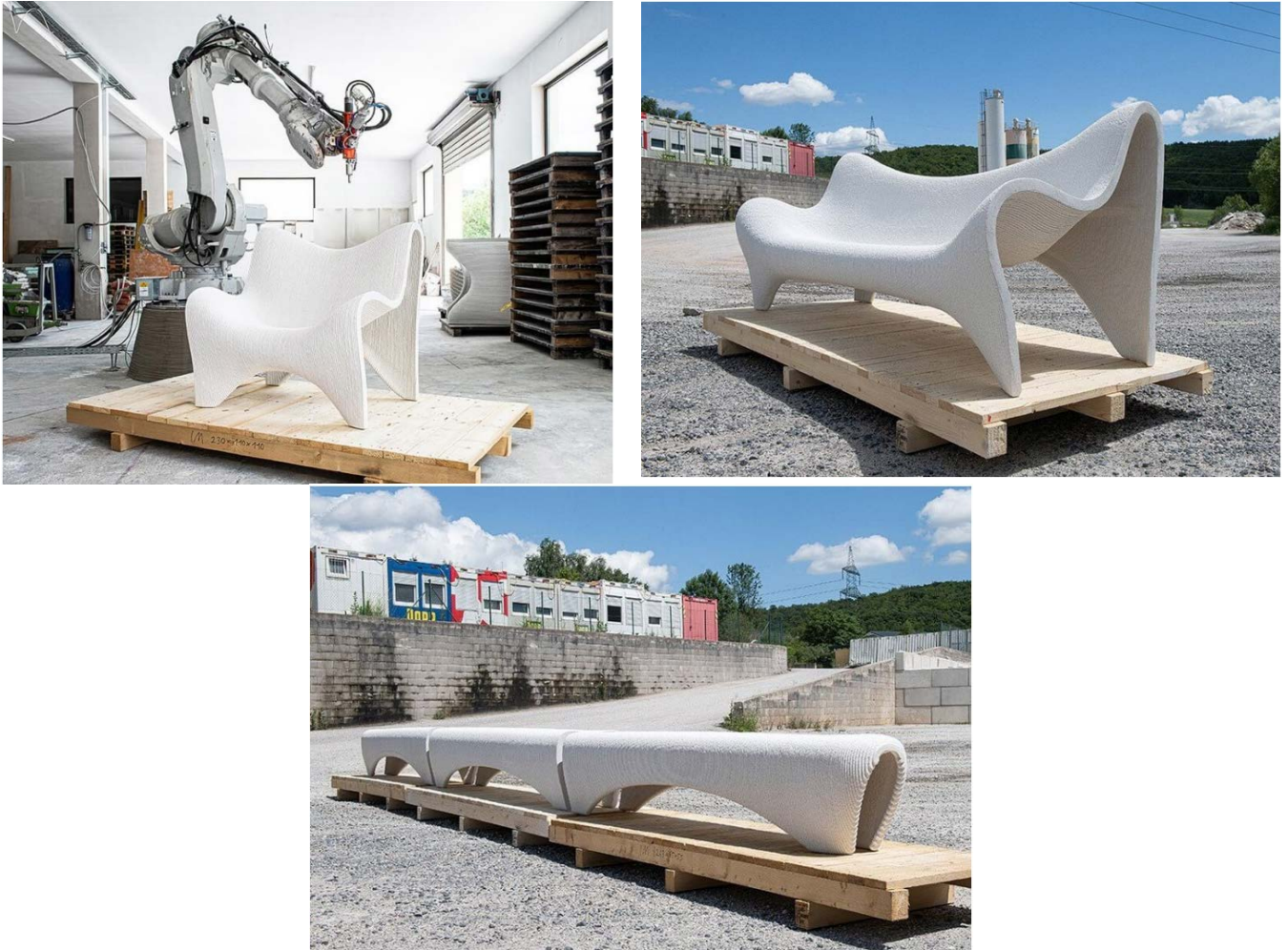
Fig. 13 3D printing concrete furniture (Philipp Aduatz 2020).
