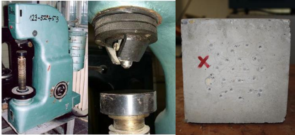
Fig. A-2 Brinell hardness tester (left); Steel ball indenter head (middle); Results of the Brinell-hardness test in practice on a concrete sample (right)
