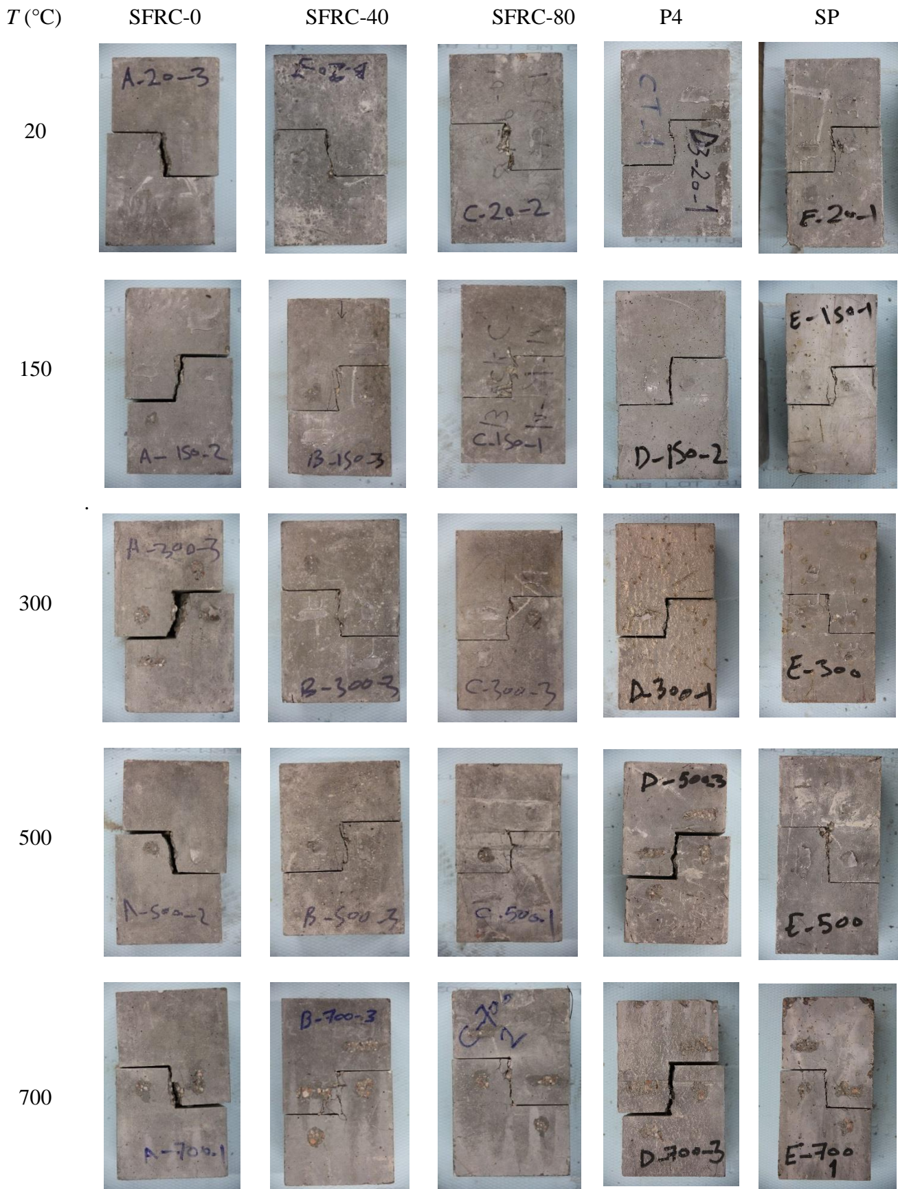
Figure 4.33: Different failure modes of the one-year old specimens after push-off loading tests
