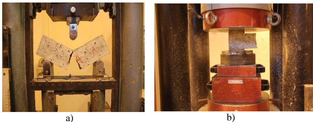
Figure 3.9: Preparations for compressive and flexural strength tests, a) flexural test and b) compressive strength
