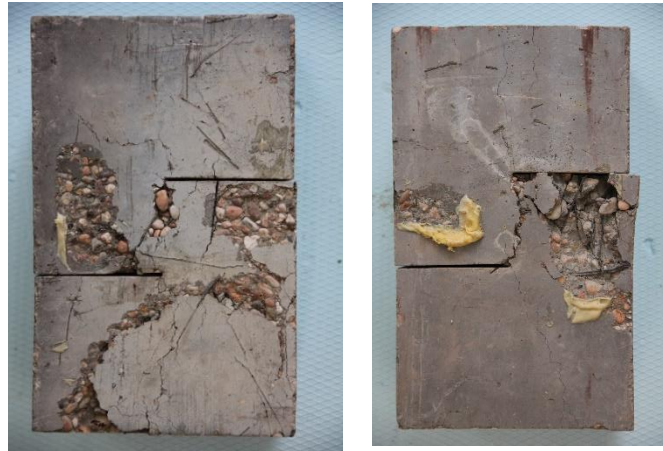
Figure 4.6: Partial spalling for some of the cocktail specimens (28-days old) at 700 °C.
